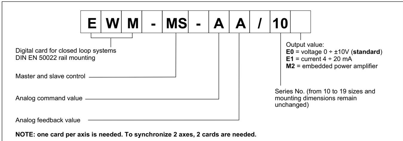
The structure of the synchronisation controller was deduced from our positioning modules. The positioning function is controlled by target position of the axis (input PIN 13) and by the actual position of the axis (PIN 14). With input PIN 6 (normally the sensor of the master axis) the actual position of the other axes is given to the module. In case of two axes, the position information can be linked crosswise from PIN 14 to PIN 6.
