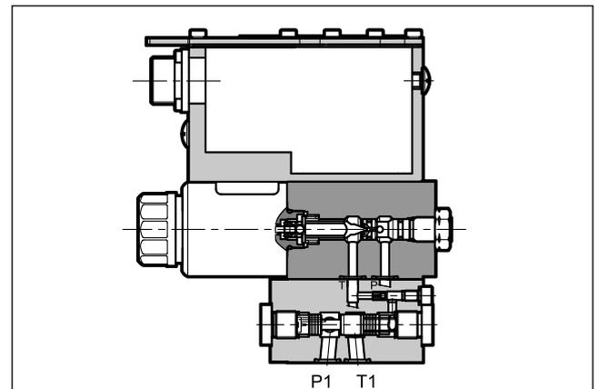
— The PRE3G valve is a pilot operated pressure control valve with electric proportional control and mounting surface in compliance with ISO 4401 standards, controlled by an integral digital amplifier.
