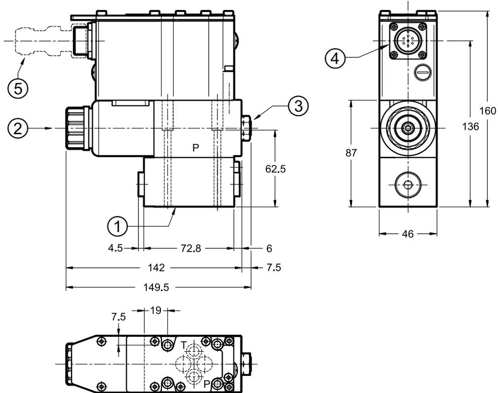
**NOTE:** at the first start up, or after a long period of no use, it is necessary to vent the air through the breather (3) placed at the end of the solenoid tube.
