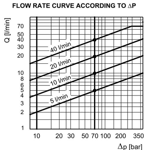
Typical flow rate curves at constant  $\Delta p = 70$  bar P-T according to the reference signal.
