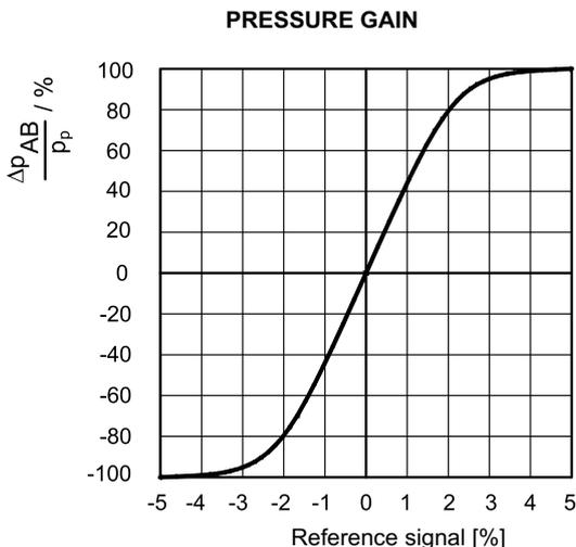
The diagram shows the valve pressure gain, expressed as % of the ratio between the port pressure variation in A or B ( $\Delta p_{AB}$ ) and the P system pressure, according to the reference signal. In practice, the pressure gain states the valve reaction towards external disturbances aimed at changing the actuator position.
