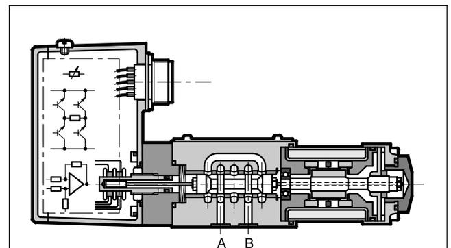
— The DXJ3 valve is a four-way servo-proportional valve where the spool moves inside a sleeve. This valve has a direct drive with a linear force motor resulting in high dynamic performances which are independent of system pressure. The spool position is controlled by a linear transducer (LVDT) with closed loop which ensures high precision and repeatability.
