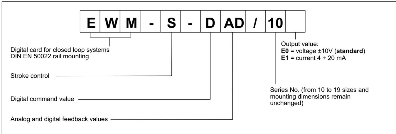
The card EWM-S-DAD is an evolution of an analog model (EWM-S-AD). The customer can choose between two sensor types: analog or digital and the communication with the PLC is via Profibus DP.
