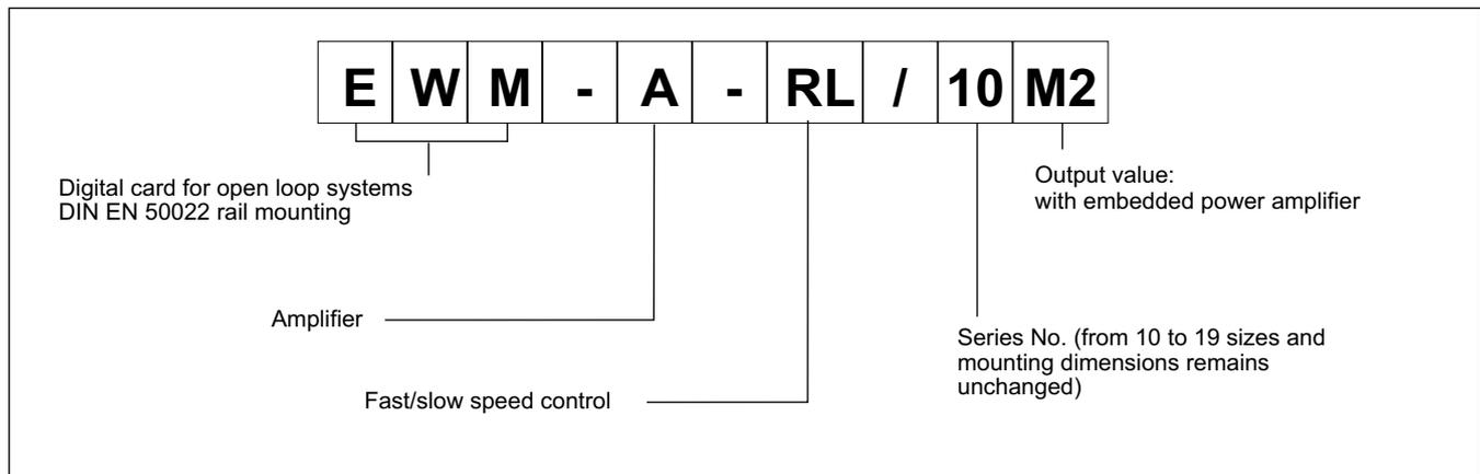
The power amplifier is controlled by an enable input and three switch signals. Therefore 8 demand values can be activated binary.
