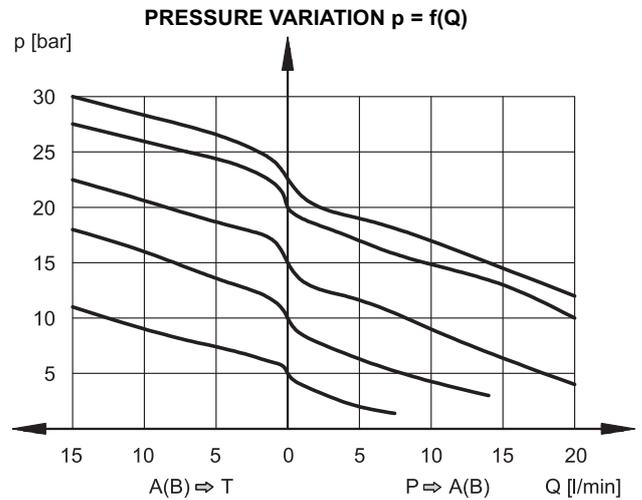
The curves have been obtained with inlet pressure 100 bar.
