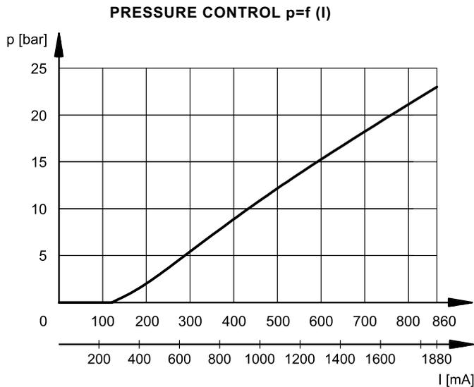
SA and SB versions pressure regulation is less than 0.5 bar.
