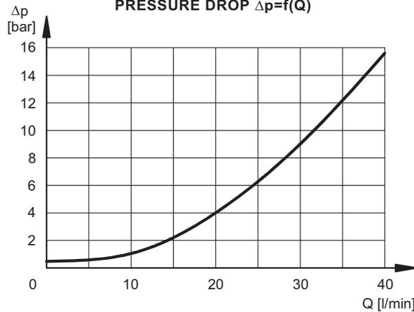
Pressure drop with free flow B → A through check valve.
