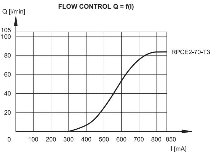
Typical flow control curves for flow rate E→T, according to the current supplied to the solenoid.
