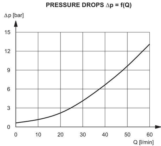
Pressure drops with free flow U → E through check valve.
