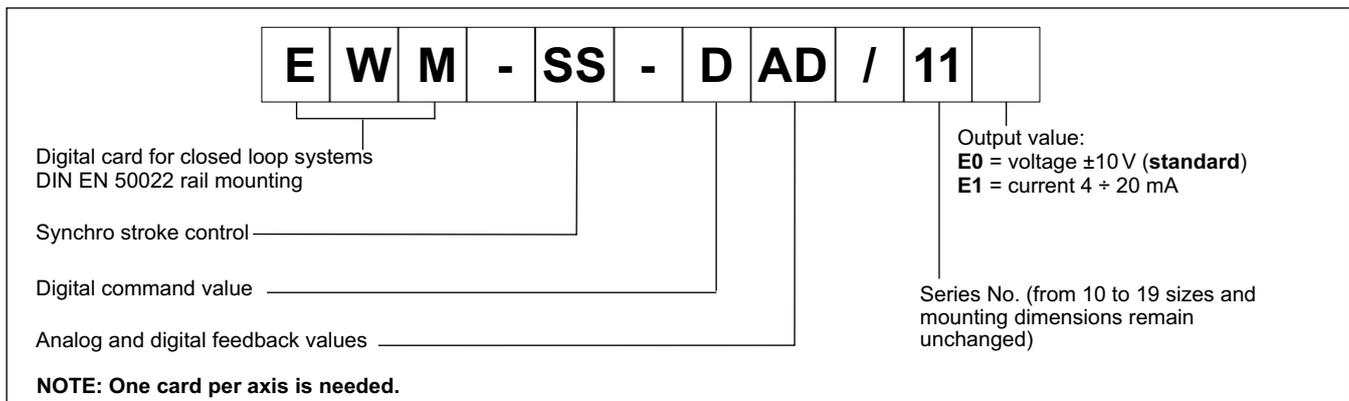
This electronic module is developed for controlling of hydraulic drives in synchronization. The communication with the PLC is solved by a standard Profibus DP interface.
