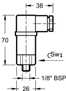
This indicator is a pressure switch sensitive to the filter input pressure, which switches an electric contact when the filter element has reached the clogging limit.
