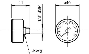
This indicator is a pressure gauge sensitive to the filter input pressure.
